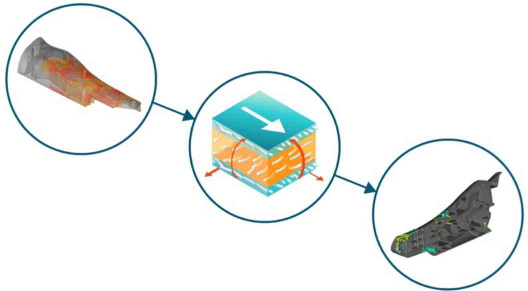
The simulation of the injection molding process provides the fiber distribution that is considered in the material property to improve the prediction quality of the structural assessment of the part.
