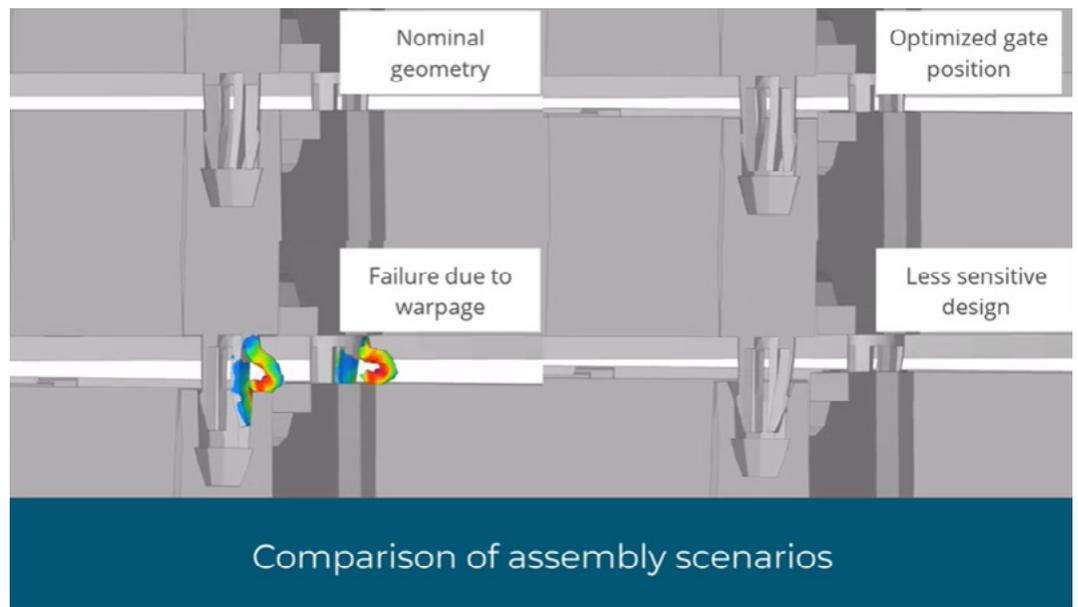
To ensure correct assembly, the gate positions for parts fitting together can be optimized to give similar warpage and shrinkage. In parts with unmatched gates, analysis of the assembly process using multiscale material properties can identify cases of potential pin connection failure, causing pins to be crushed during assembly. By increasing tolerances, these costly assembly issues can be avoided.
