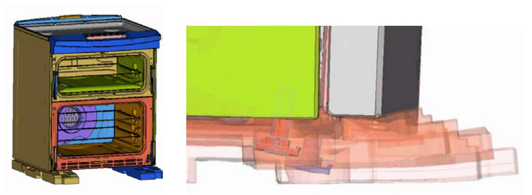
Mabe uses Altair structural analysis tools to predict and prevent damage during shipping and handling.
