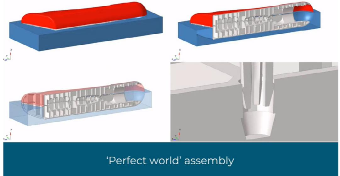
Structural analysis of a medical auto-injector during part assembly.
