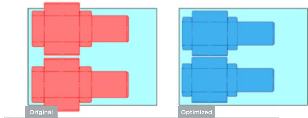
Additionally, a smaller box made it possible to fit more units per pallet. This makes it easier to ship the same quantity of product using fewer containers and fewer trucks, reducing both carbon footprint from the material reduction as well as shipping and logistics improvements.
