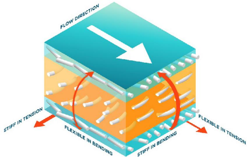
Process dependent fiber orientation and resulting material behavior: Depending on the plastic used, the geometry of the component and the process conditions, a three-layer distribution of the fibers occurs. On the edge of the component, the fibers tend to lie in the direction of molding, while in the center the orientation is transverse.
