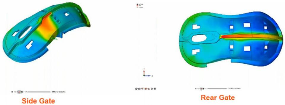
Filling simulation to quickly evaluate different injection gate positions.
