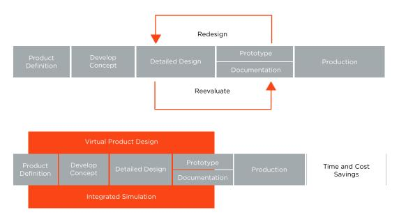
Whereas virtual product design applies integrated simulation tools across the whole design process which means that both design and process variables can be investigated together and optimized much earlier. Fewer physical prototypes, with the physical testing needed for each, significantly reduces the time and cost to market meaning fewer scrap parts, less waste, lower tooling costs, less energy while also providing confidence of fewer in-service failures.
